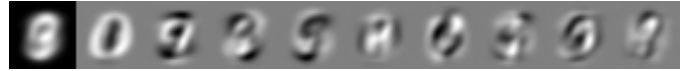
Fig. 2. The mean values (left) and first 9 principal components of the MNIST dataset. (Greyscale ranges have been rescaled for maximum visibility.)
